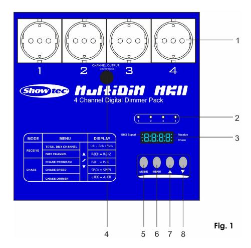
1) Channel Output: 8x 3-prong grounded Edison sockets.10 A per channel, total 20 A max.
